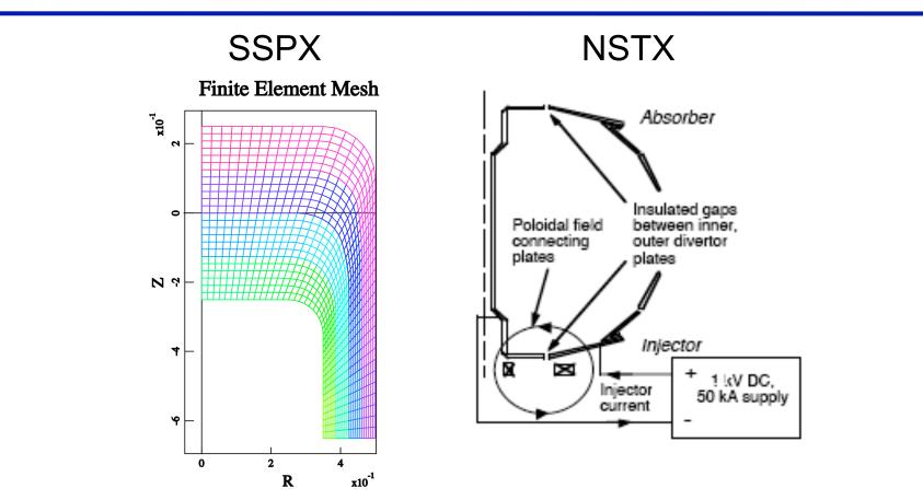
The SSPX grid efficiently mapped the "gun" region into the spheromak volume
